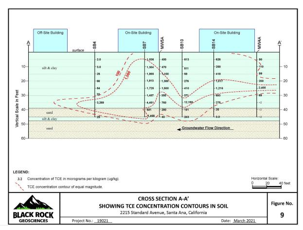
Diceon cross section, showing dynamic vertical understanding of contaminants' concentrations at different strata of the geology and hydrology.
