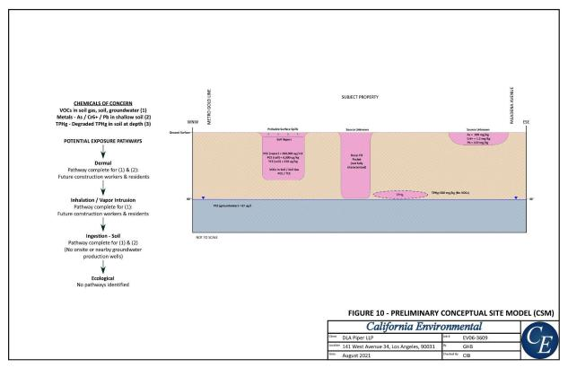
Avenue 34 cross section, with arbitrarily delineated rectangles standing in for confirmed contaminant depths, and acknowledgements that characterization is incomplete.
